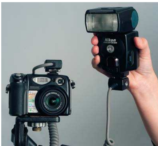
Figure 16.7 You can use your flash as a studio light replacement and can free the unit from its hot shoe base by using an extension cable. The cable maintains a link for all the flow of exposure and triggering information, whilst allowing the photographer to position the flash head away from the camera body.
